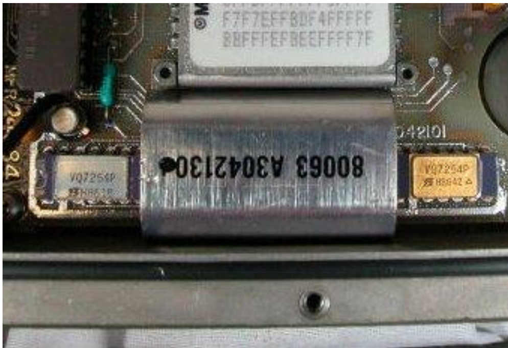
SILICONIX 7254 Drive Transistors marked VQ7254P in Military Bubble Memory Unit
